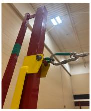
THE CARIBINER ON THE TOP CHAIN CLIPS DIRECTLY TO THE METAL LOOP ON THE POST.
